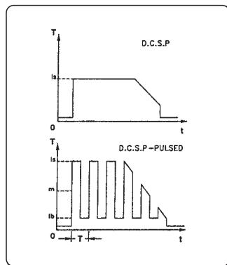
**D.C.S.P.-Pulsed (Direct Current Straight Polarity Pulsed)**
